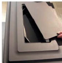
In order to have a better access to the smoke channels, the baffle plate can be taken out or pushed toward the firing door.
